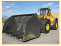
handled: dry recycled chip which is made from anything from a scrap pallet to an old wardrobe, and wet chip which is made from newly felled tree logs. Dry chip tends to hang in the air and gets sucked into the air filters of the big machines. Wet chip on the other hand falls to the ground quickly and causes no problem to the air filters.
