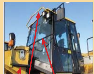
Upper and lower grab rails and step installed
