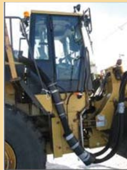
No ladder for access
