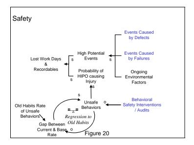
As shown in Figure 20, the level of risk in the environment is highly dependent on the reliability of the plant. Every unplanned outage presents a risk. In some plants, this can be the risk of fire or explosion. In other plants it can mean flying debris. In all cases, failures mean having to take some corrective action and corrective action is inherently dangerous.
