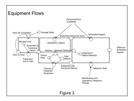
The first example, shown in Figure 3, is the backbone of the entire model. In it the "equipment perceived good" stock represents all of the equipment without any known defects. If a defect is detected in that equipment, then its' status moves to the category of "equipment with perceived defects" stock. Defect detection can be done through a formal inspection, by operators conducting rounds or by a root cause being detected during a repair or proactive intervention.
