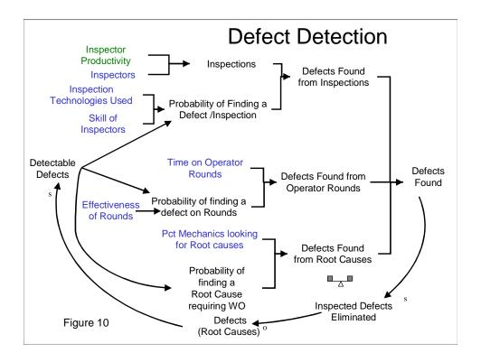
There are three primary ways that defects are detected proactively and are put into the scheduled maintenance process: formal inspections done by the inspection specialist, operator rounds and root cause analysis.
