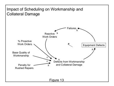
By reducing failure events, scheduled work reduces collateral damage from failures and reduces rushed reactive repairs that are inherently lower in workmanship. The assumption in our model is that reactive repairs are 20% more likely to introduce an error due to faulty repair than a scheduled repair.
