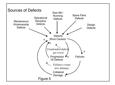
Unfortunately, defects breed more defects. As seen in the "Unattended defects get worse" loop, defects tend to grow worse over time if unattended -- today's defect that has little or no operational consequences will most likely be the cause of tomorrow's catastrophic failure. Failures also create defects by causing collateral damage.
