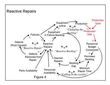
The next example, in Figure 4, shows the process for when equipment fails reactively and goes through a "reactive repair" loop. Repairs are completed as personnel and parts become available, and the symptomatic cause of the failure is eliminated.
