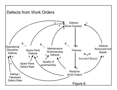
In the course of repairing defects, poor workmanship, poor spare parts quality and poor practices in startup and shut down can lead to new defects and new problems. Often these defects will show up as "infant mortality" failures where a system will fail several times in rapid succession after a repair. Figure 6 shows these unintended consequences of doing repair work. The rate at which defects are added through repair depends on the skills, standards and culture of the organization.
