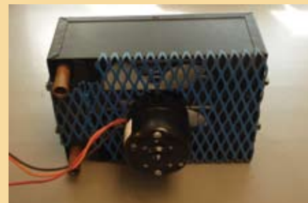
After fan guard installation
